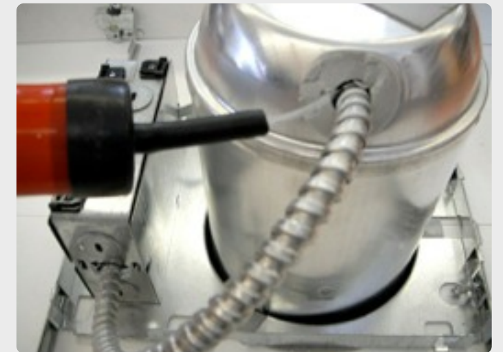
A recessed light can from the attic. The smoke from a red and black puffer is being sucked into the wiring hole during a blower door test.
