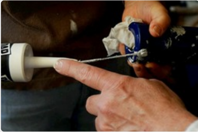
Puncture the inside membrane with the wire on the caulk gun or a long nail.
